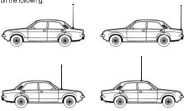
**Roof Mount** - In this position the antenna radiates equally in all directions. Since the normal 1/4 wavelength whip antenna is too long for roof mounting on a veicle, the antenna is shortened and loading coil is used to provide the proper electrical lenght. Our fiberglass roof mount is a good durable antenna.
